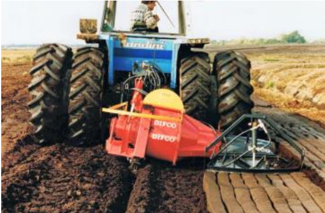
Plate 4-18 Process of extracting bin sod. The peat is macerated, extruded into sods and cut with trailing discs (source: BnM).
