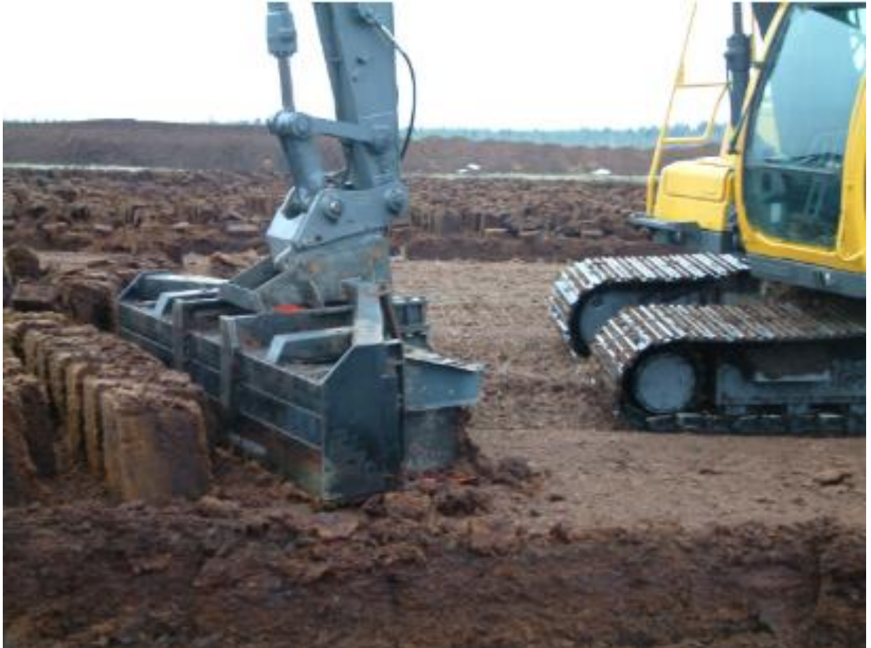
Plate 4-37 Sod Moss cutting attachment attached to a digger (source: BnM)
