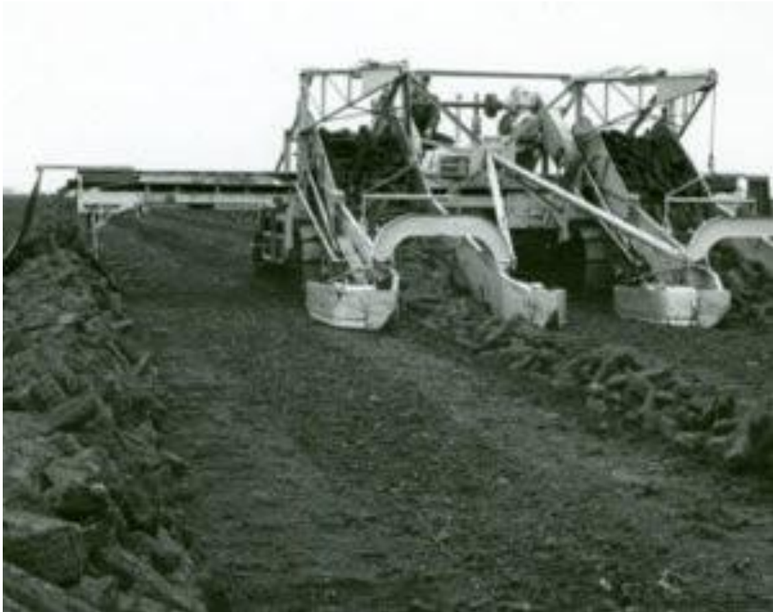
Plate 4-22 Sod turning machine (source: Living History)
