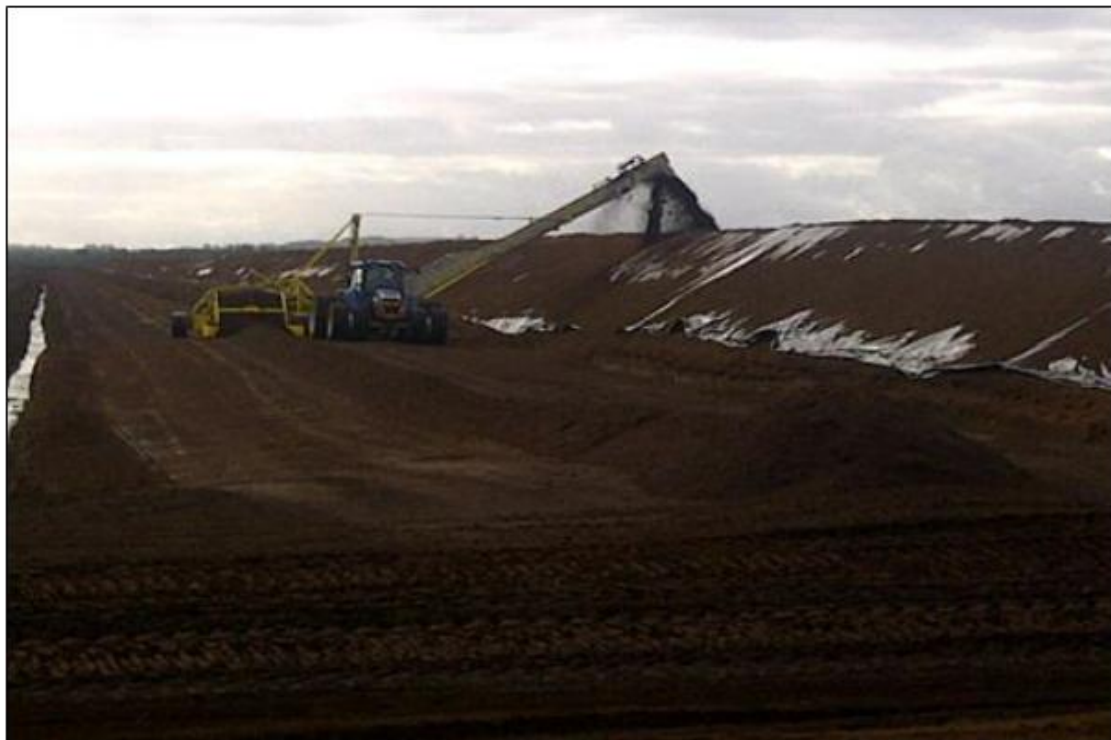
Plate 4-15 Process of Stock Protection, showing a layer of milled peat being spread over polythene sheeting to anchor the sheeting in place (source: BnM)
